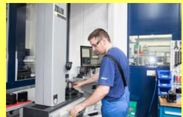
»venturion450/8« for measuring and inspecting highly complex tools at VAT in Haag, Switzerland
