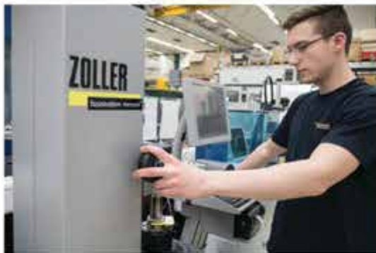
The »venturion 450«, a CNC-driven tool presetting and measuring machine from Zoller.
