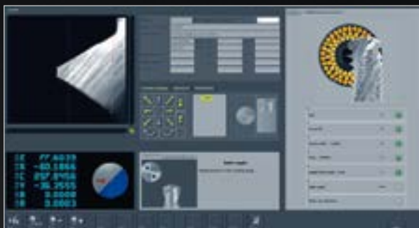
Measuring Program for Thread Milling Cutters in Incident Light
