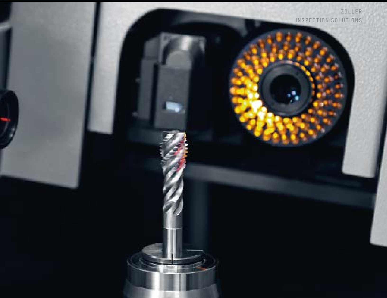
Measuring Program for Thread Milling Cutters in Incident Light
