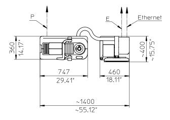
Note: P air connection E electronic connection
