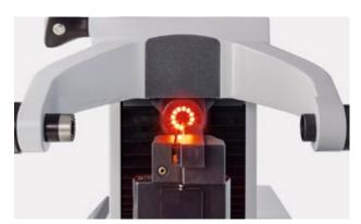
Center height measuring camera on the optics carrier with LED ring light
