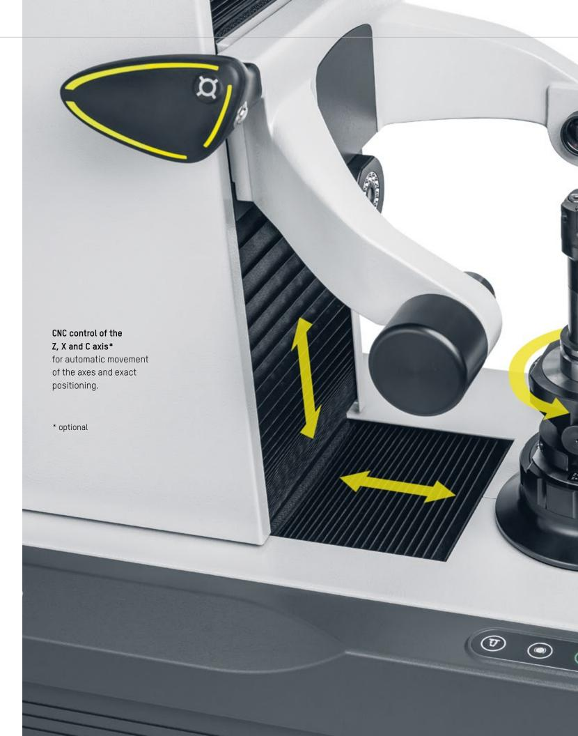
Autofocus\* to automatically focus the cutting edge for accurate measuring results.
