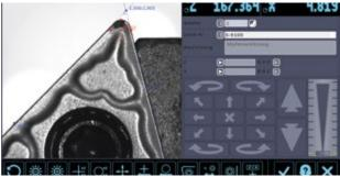
Cutting tool inspection in »pilot 1.0« software
