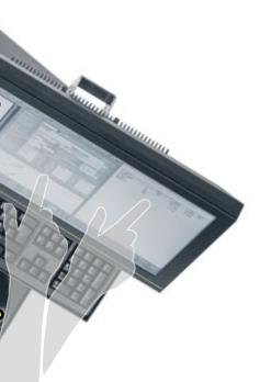
Adjustable control unit – can be tilted, adjusted in height and swivel. This allows every operator to optimally adjust his or her workplace with just a few hand movements.
