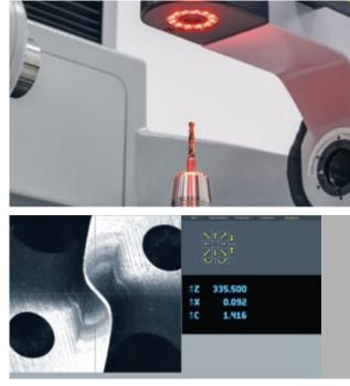
The face of the tool is displayed and measured in the »metis« tool analysis software.
