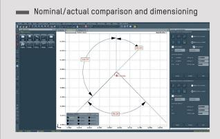
This function enables a nominal/actual comparison with DXF ideal contours and automatic dimensioning of the section via the contours of the cutting edge.
