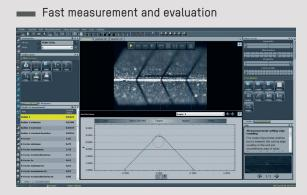
One can choose between a live image or a graphic display. The live image facilitates positioning, alignment and inspection of the cutting edge.
