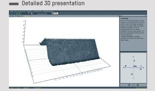
The cutting edge can be displayed in different modes: texture presentation for immediate detection of possible surface indentations and surface quality.
