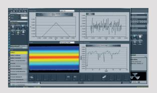
The cutting contours are displayed in a clear manner. At the same time, the evaluated chipping and radius contour are displayed.
