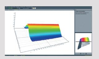
The topographic representation shows the height contours of the cutting edge preparation at a glance.
