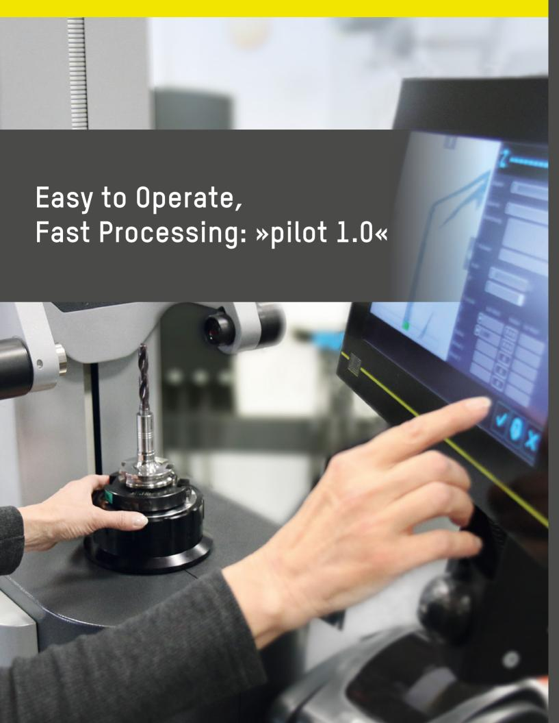
The new image processing technology »pilot 1.0« offers all functions for presetting and measuring standard tools quickly and easily. For instance "Automatic cutter shape and measuring range detection", navigation system »compass«, "projector function and cutting edge inspection", »cris360°« to determine the effective cutting area of tools, and a clear representation of the tool cutting edge on a 13.3" panel PC.
