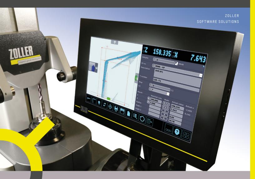
Simple and Fast Measuring and Presetting of Standard Tools
