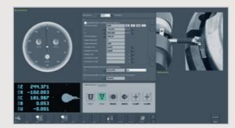
Measurement and compensation of concentricity and run-out at the hub diameters of the tool.
