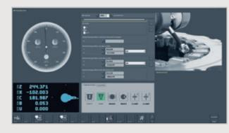
Entry of freely definable parking and safety positions to optimize measuring procedures for maximum safety.
