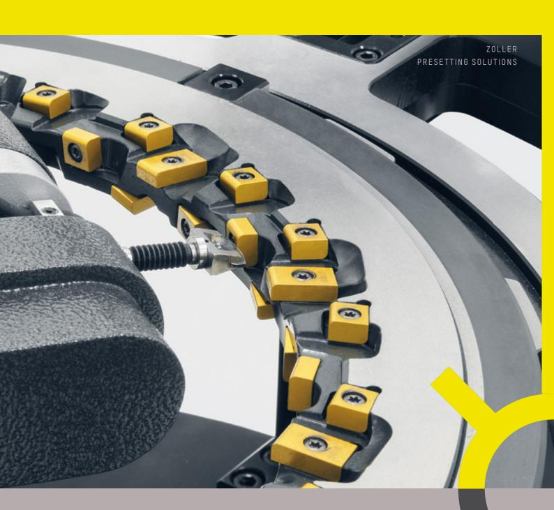
The Measuring Machine for Crankshaft Cutters with Internal Tool Cutting Edges
