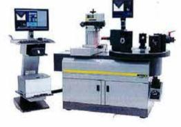
light and vertical lighting contexts. This makes it easy to check and measure all tool geometries and to log results in accordance with applicable regulatory directives.
