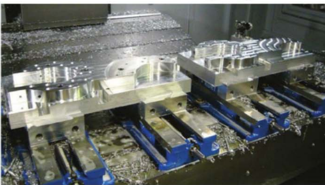
A pair of saw guides in process. The new Sharp Industries Box Way Vertical Machining Center SV-6332SX allows the fixture of multiple parts on the table, which results in a longer unattended cycle time. This is a key concept to allow a single operator the ability to run several machines at once. With automated probing as part of the setup, the operator can mount the raw stock or parts in a fixture, hit cycle start and walk away, returning only to remove the parts and fixture for the next set. The operator is free to go to another machine and repeat the same process for a different operation or part.
