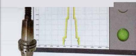
matches the tool originally used for the simulation. The tool's real, actual contour is recorded while being rotated, thus simulating the actual machining process.
