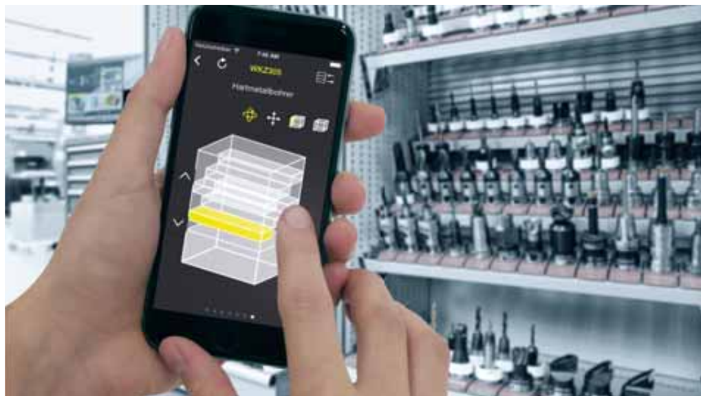
With the TMS Tool Management Solutions app SILVER version, tools can be moved into and out of a selected storage location.
