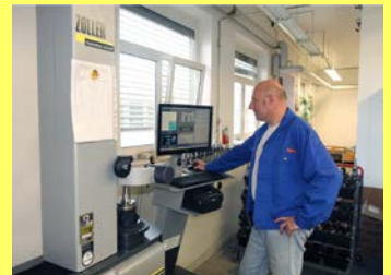
The ZOLLER solution for GMN Paul Müller Industrie GmbH & Co. KG: tool presetter machine with TMS Tool Management Solutions
