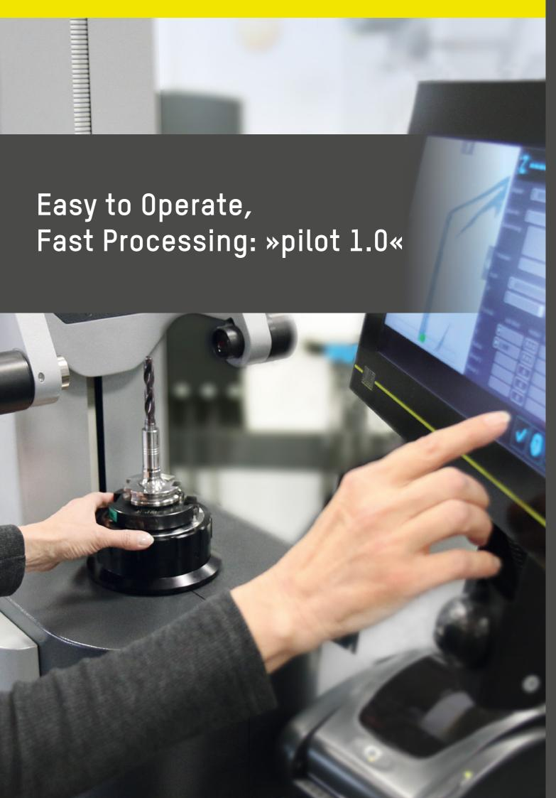
The new image processing technology »pilot 1.0« offers all functions for presetting and measuring standard tools quickly and easily. For instance "Automatic cutter shape and measuring range detection", navigation system »compass«, "projector function and cutting edge inspection", »cris360°« to determine the effective cutting area of tools, and a clear representation of the tool cutting edge on a 13.3" panel PC.
