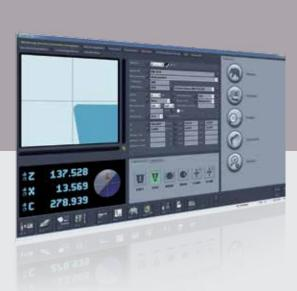
Tools released for presetting are compiled in a list and can be preset and measured at the push of a button. Then they are released for production.
