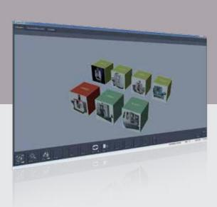
The »flash« software module automatically queries the tool life per machine independently of the operator. Colors symbolize the current status of the tool life. Tools whose life has expired or whose warning limit has been reached, can be selected and released for recommissioning.
