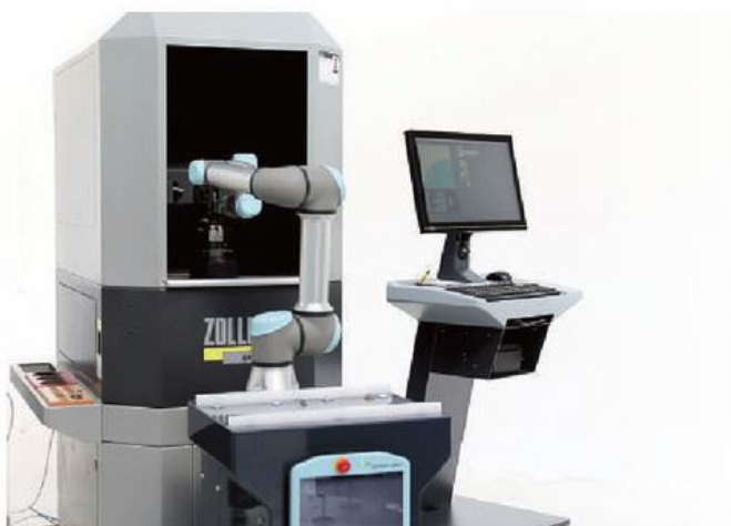
AutoComp ensures tool quality in lights out production
