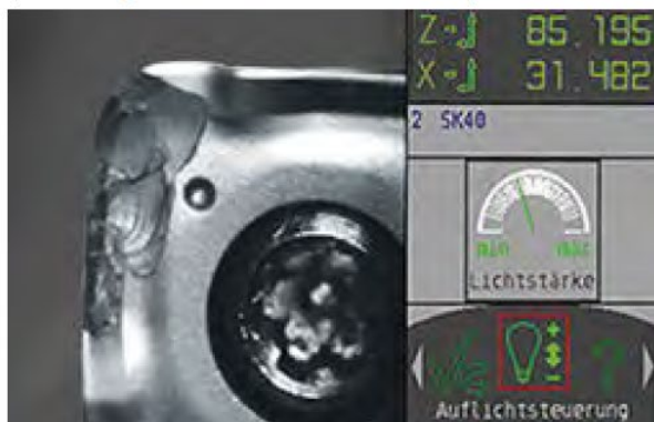
Cutting edge inspection – 12-fold magnification of the cutting edge in incident light for quality control (option)
