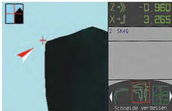
Compass needle for simple camera positioning to measure nominal values (option)
