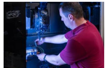
The third axis, the Y axis on the ZOLLER »hyperion« measuring machine, makes it possible to fully measure turning tools on multi-piece holders
