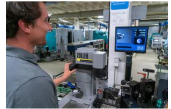
The third axis, the Y axis on the ZOLLER »hyperion« measuring machine, makes it possible to fully measure turning tools on multi-piece holders
