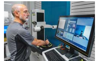
Thanks to the graphic warehouse interface offered by ZOLLER Tool management, a SIM employee can remove the tool he needs efficiently from the Hänel lift tool storage system.
