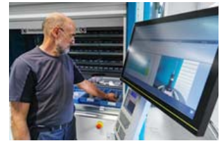
Thanks to the graphic warehouse interface offered by ZOLLER Tool management, a SIM employee can remove the tool he needs efficiently from the Hänel lift tool storage system.
