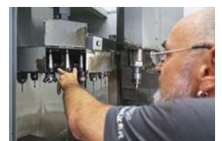
Then measured data is transferred to the machine through the network via control-ready data output. After being read in, it is directly ready for use by the machine.
