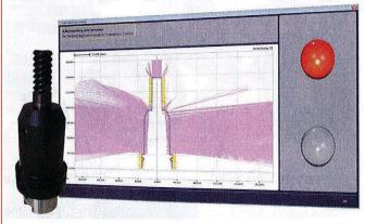
the starting point and measures the contour during rotation. An actual/nominal comparison is displayed along with the results of the collision check. A green light means that the machining processes can be performed; a red light indicates a collision. The module is available for all Zoller CNC tool presetter and measuring machines.
