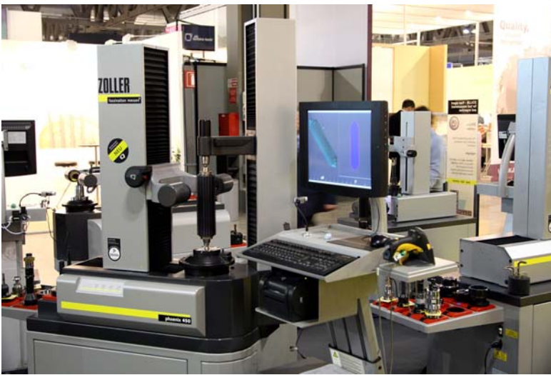
Picture 4: The ZOLLER »phoenix«: \mu -precise presetting and measuring of reamers.
