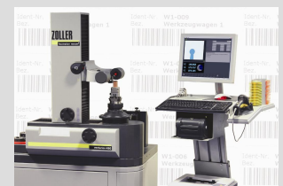
Caption: ZOLLER »cockpit« designed for working with barcodes. In the picture, it is equipped with a barcode reader, printer and Tool Tags as well as the Tool Tag holder.
